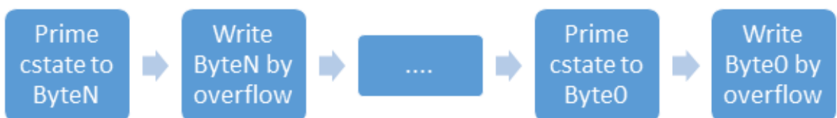
Flow for writing arbitrary sequence of bytes after the buffer
