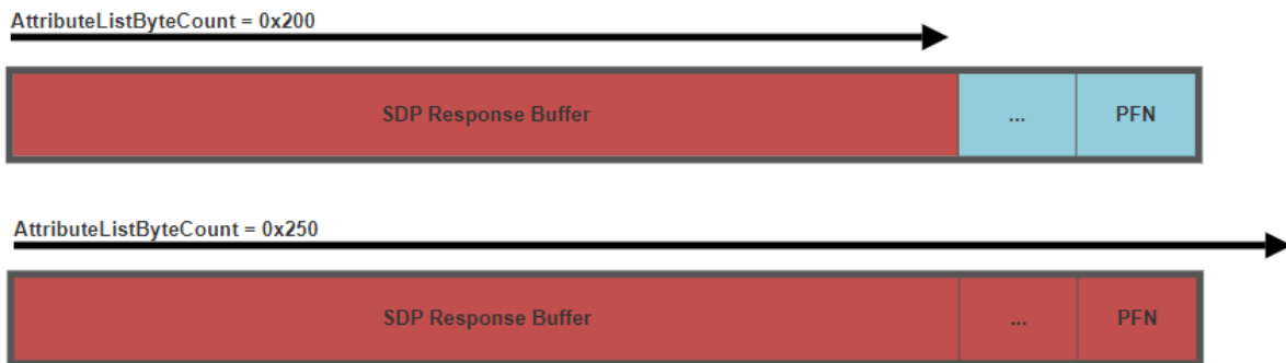
Comparison of two overflows exploiting Hell2CAP; the difference is the AttributeListByteCount sent in each request
